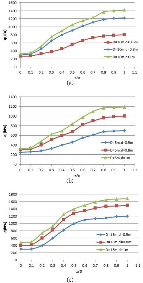
**Figure 6:** Variation of ultimate bearing capacity ( $q$ ) with the ratio of granular-fill depth to footing diameter ( $z/D$ ) for  $L=0.5D$
