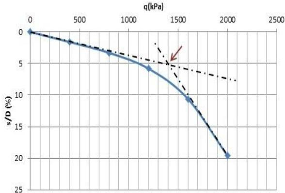
**Figure 5:** Typical determination of the ultimate bearing capacity value
