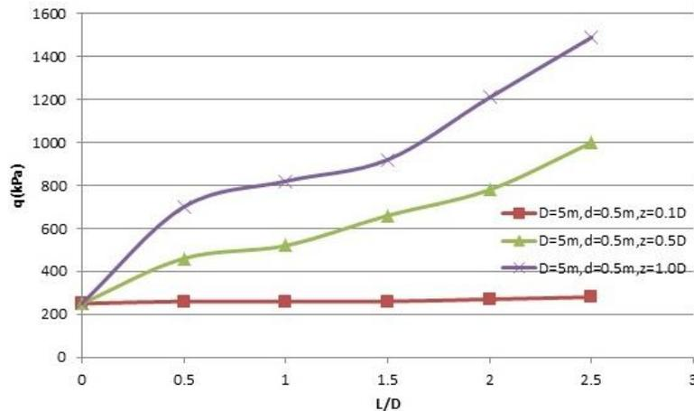
**Figure 9:** Variation of ultimate bearing capacity ( $q$ ) with the ratio of granular-fill length to footing diameter( $L/D$ )
