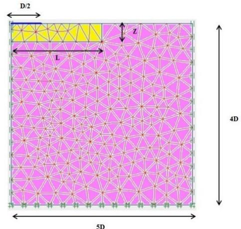
**Figure 4:** The typical finite element mesh used in the study
