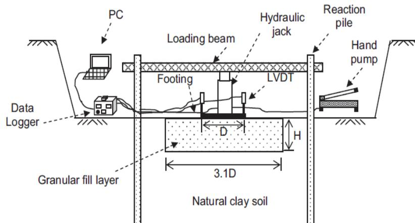
**Figure 1:** The general layout of the test setup by Ornek et al. (2012)
