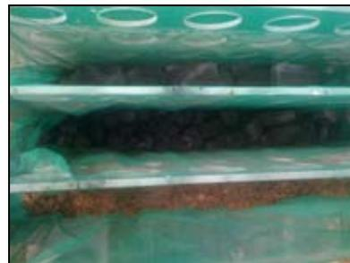
**Figure 3:** Arrangement of Filtering Materials
