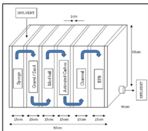
**Figure 4:** Illustration of mechanism of biofilter system
