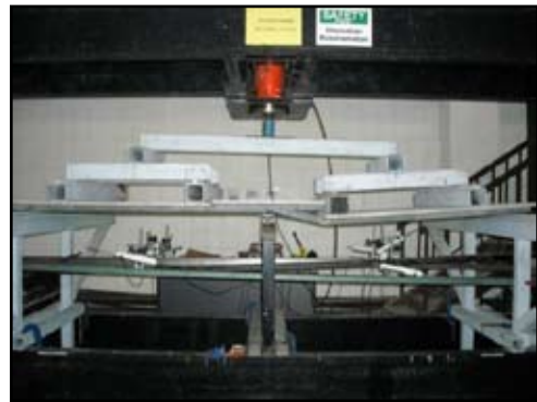
Figure 5: The semi-continuous panel loaded until failure
