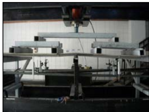
Figure 6: The continuous panel loaded until failure
