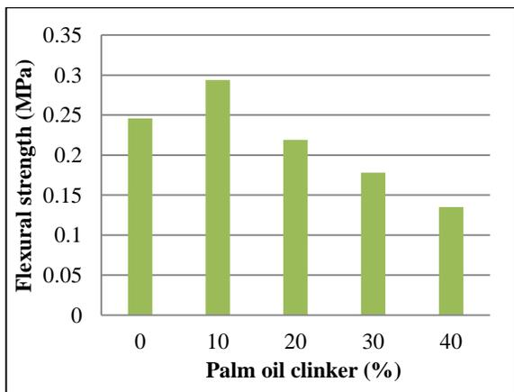
Figure 9: Flexural strength result up to 28days
