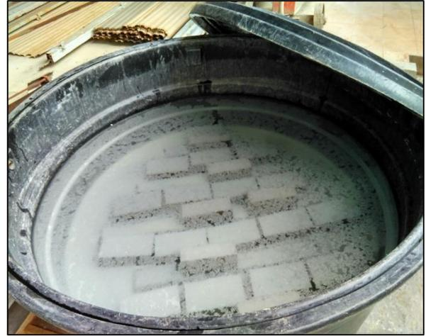
**Figure 6:** Specimen subjected to water curing
