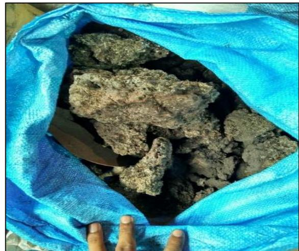
Figure 3: Palm oil clinker chunks before grinding
