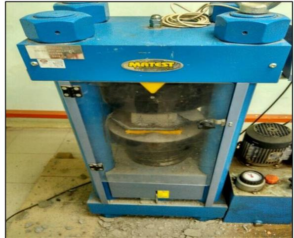
**Figure 7:** Compressive strength test in progress
