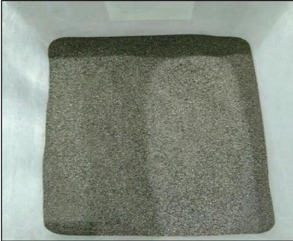
**Figure 4:** Fine palm oil clinker after grinding
