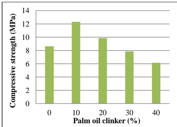
Figure 8: Compressive strength result up to 28days
