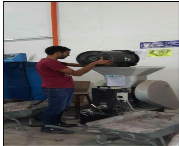
Figure 2: Palm oil clinker pulverizing process
