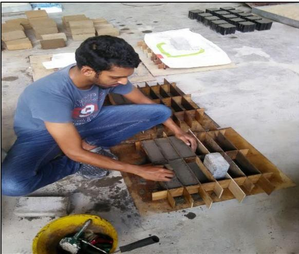
**Figure 5:** Casting of brick specimen
