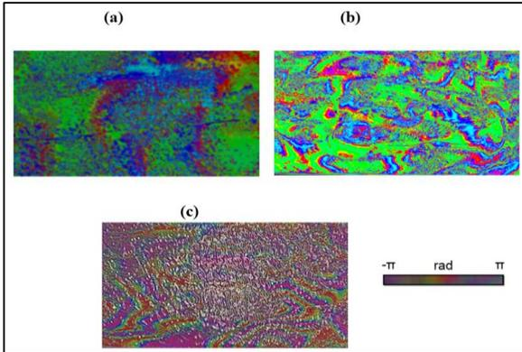
**Figure 5:** Phase unwrapping (a)2-D;(b)3-D; and (c) 4-D
