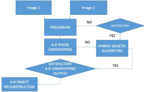
**Figure 3:** Hologram interferometry procedures
