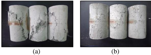
**Figure 4:** Mode of failure for (a) NC and (b) TCRSFC7
