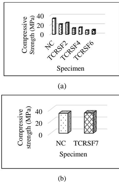
**Figure 2:** Compressive strength of concrete specimen (a) 0.55 water cement ratio and (b) comparison for 0.55 water cement ratio (NC) and 0.50 water cement ratio (TCRSFC7)
