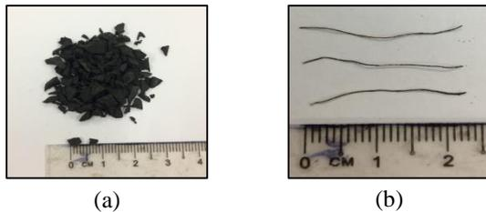
**Figure 1:** (a) Crumb rubber and (b) Steel fiber
