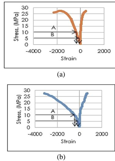
**Figure 3:** Stress-strain curve of (a) NC and (b) Stress-strain of TCRSFC7, A is secant modulus and B is dynamic modulus.
