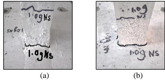
**Figure 5:** Damage of column specimen after seismic shaking table test. (a) NC (b) TCRSFC7
