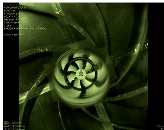
**Figure 5:** Snapshot picture from high-speed camera showing rotation of small fan inside the tower.
