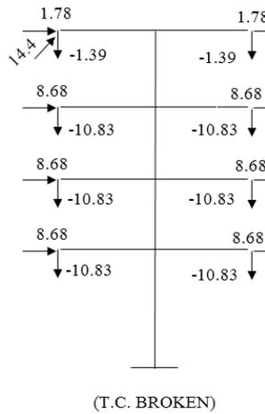
**Figure 5:** Top Conductor Broken
