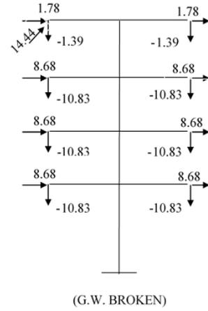
**Figure 3:** Ground Wire Broken
