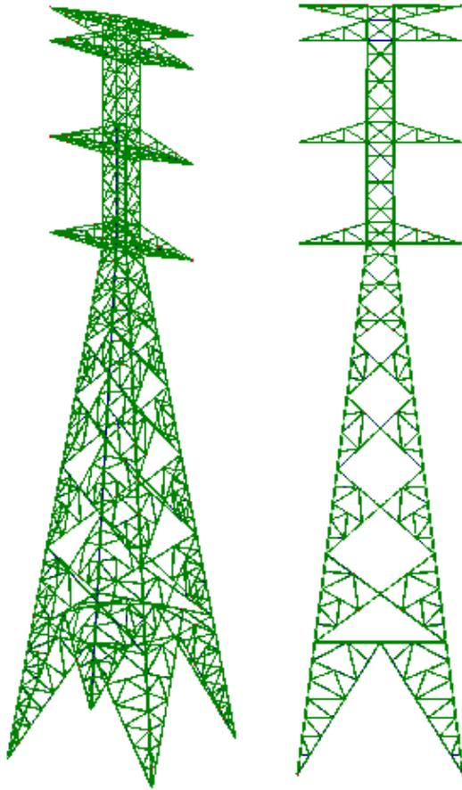
**Figure 1:** The 3D model of 275 kV OTT
