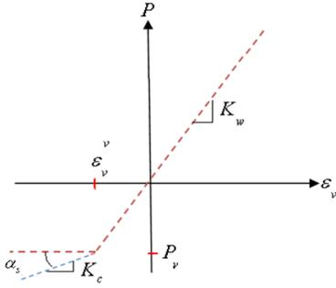
**Figure 2:**The bilinear model for cavitation
