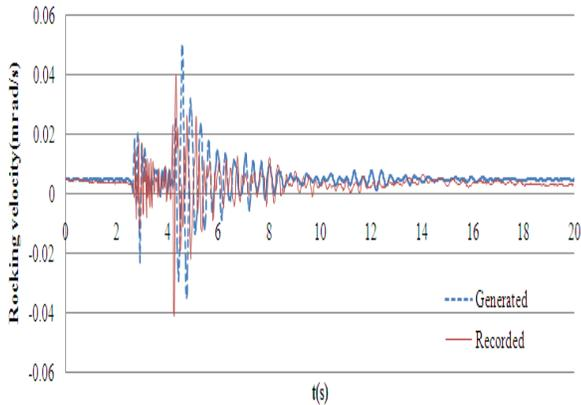
**Figure 8:** Time history of rotational velocity recorded by S-5-S sensor (Kalabet al.2012a; 2012b) and generated in this research
