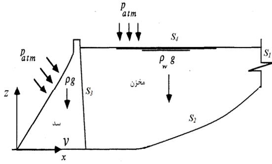
**Figure1:** The dam-reservoir system, boundaries, coordinate system and applied load
