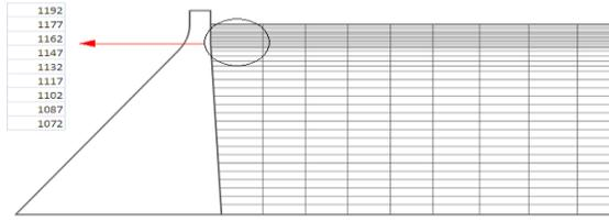
**Figure12:**Number of reservoir element on upstream face of dam
