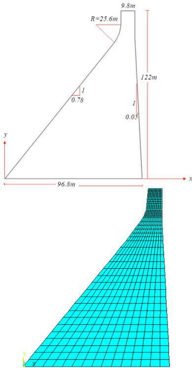
**Figure 6:** Geometrical and finite element model of Pine flat dam
