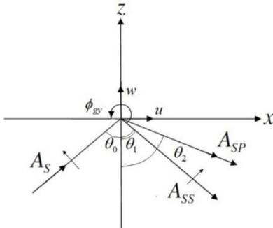
**Figure 3:**Propagation of SV wave
