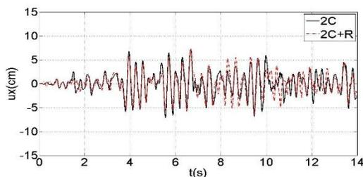
**Figure 15:** Dam crest displacement considering nonlinear behavior of water due to (2C) and (2C+R) excitations of Taft earthquake with  $SF = 3$
