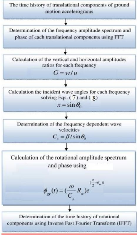
**Figure 4:**Flowchart of generating rotational component
