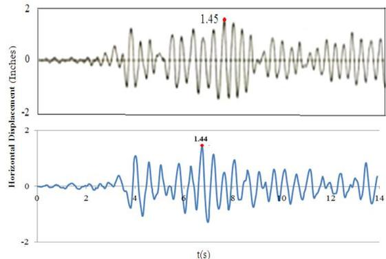
**Figure 11:** Time history of horizontal displacement of Pine flat dam-reservoir system due to S69E component of Taft earthquake, (Fenves and Chopra, 1984) and this research
