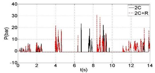
**Figure 16:** Hydrodynamic pressure of element number 1177 due to (2C) and (2C+R) excitations of Taft earthquake with  $SF = 3$
