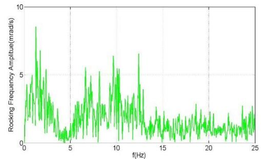
**Figure14:**Fourier amplitude of Taft earthquake rocking component with  $V_s = 385.4$
