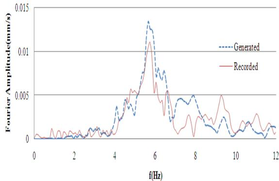
**Figure 9:** Frequency content spectrum of rotational velocity recorded by S-5-S sensor (Kalabet al.2012a; 2012b) and generated in this research
