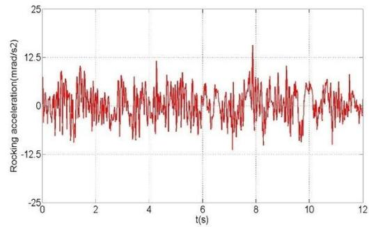
**Figure13:**Time history of Taft earthquake rocking component with  $V_s = 385.4$
