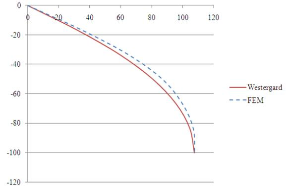
**Figure 10:** Hydrodynamic pressure on vertical upstream face of a rigid dam, (Westergard, 1933) and this research
