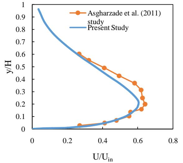
**Figure 8:** Comparison of velocity profiles with the experimental results at  $x/L=0.625$
