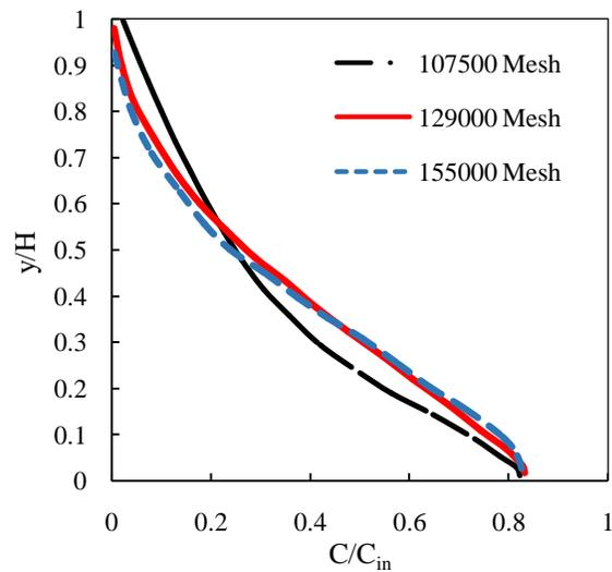
**Figure 3:** Concentration profiles for the investigation of grid independency at  $x/L=0.75$
