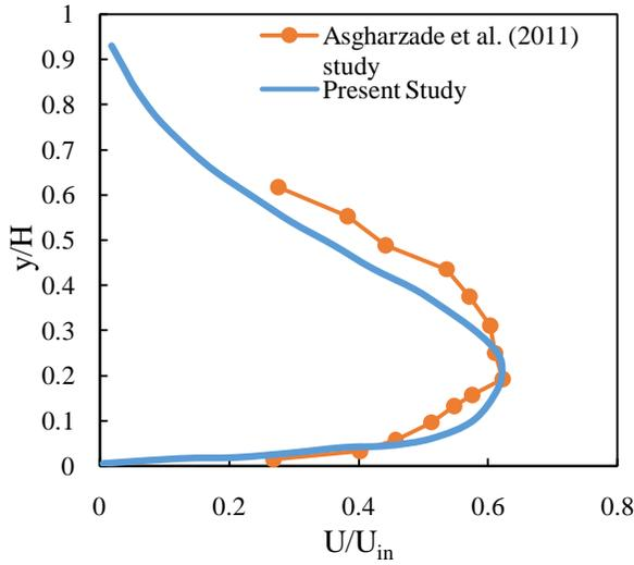
**Figure 7:** Comparison of velocity profiles with the experimental results at  $x/L=0.55$
