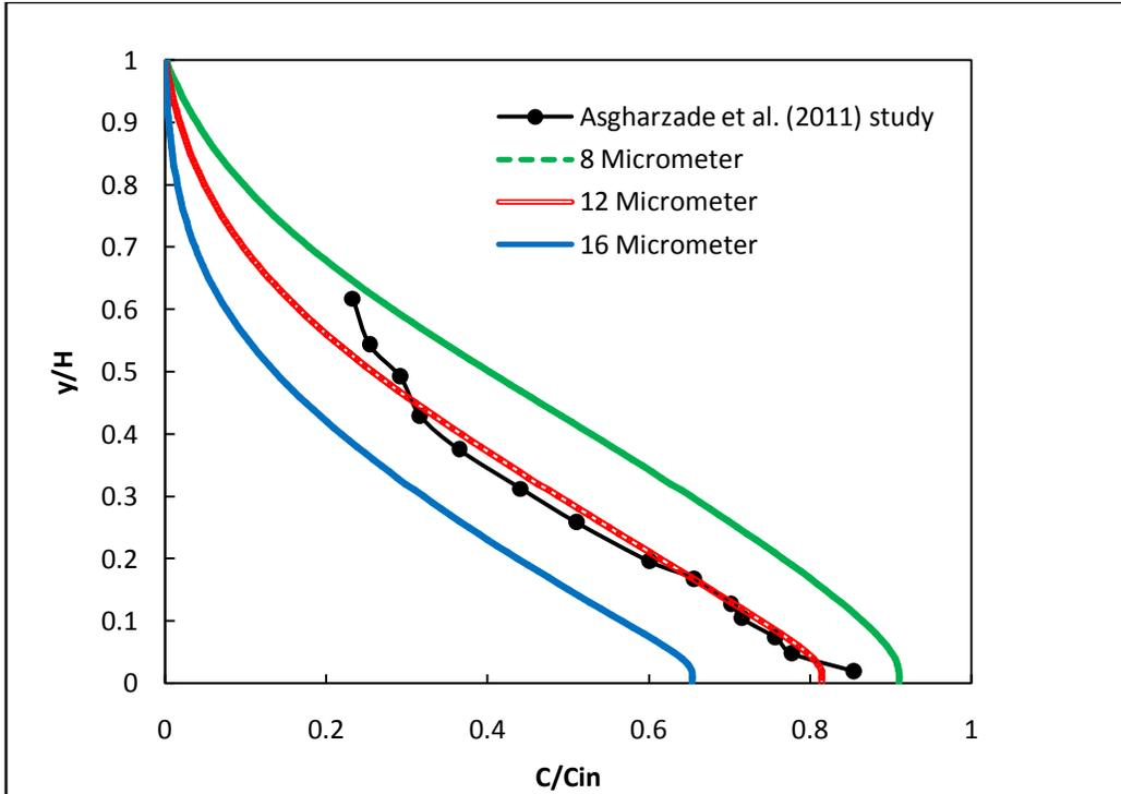
**Figure 6:** Concentration profiles at  $x/L=0.75$  for various particle sizes
