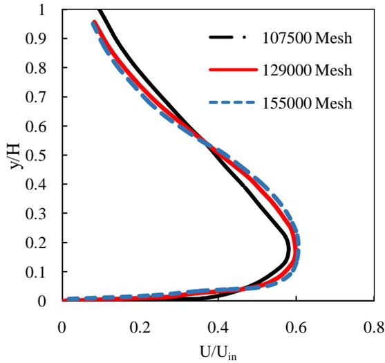
**Figure 2:** Velocity profiles for the investigation of grid independency at  $x/L=0.75$
