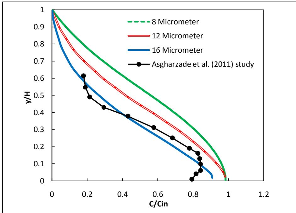
**Figure 4:** Concentration profiles at  $x/L=0.55$  for various particle sizes
