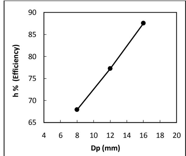
**Figure 11:** Effect of the particle size on the tank efficiency
