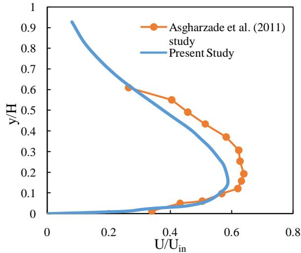
**Figure 9:** Comparison of velocity profiles with the experimental results at  $x/L=0.75$
