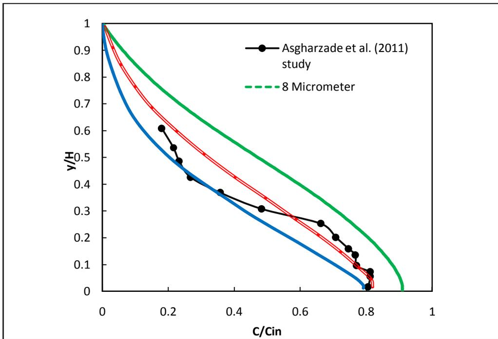
**Figure 5:** Concentration profiles at  $x/L=0.625$  for various particle sizes
