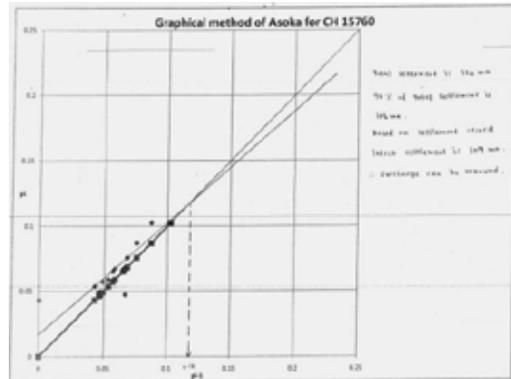
**Figure 2c:** Settlement rate using graphical method of Asoka CH 15760
