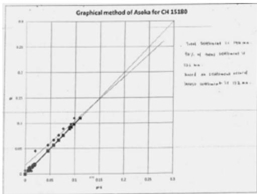
**Figure 2a:** Settlement rate using graphical method of Asoka CH 15180
