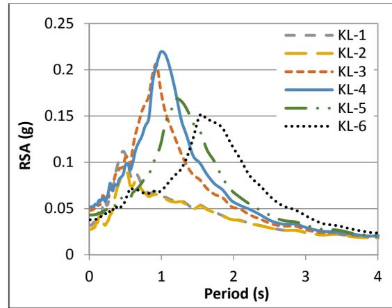
Figure 3: Mean response spectra at 5% damping
