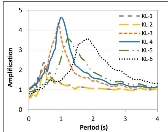
Figure 4: Average soil amplification at 5% damping
