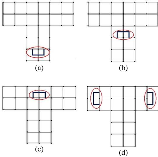
**Figure 1:** Typical plan view of T-shape building model showing shear wall position at (a) bottom wing, single (B-SGL); (b) center, single (C-SGL); (c) top, single (T-SGL) and (d) top wing at both ends (T-DBL).
