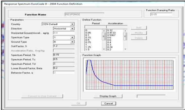
**Figure 3:** Response Spectrum Graph in SAP2000 Computer Software
